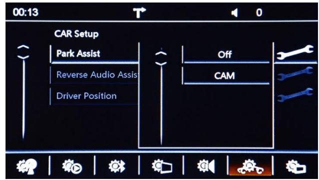
Park Assist – This is where you program the Zenec for reverse camera
