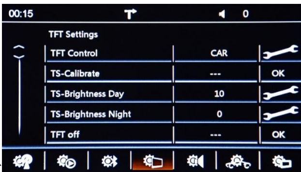
TFT Settings – This menu allows you to change the device brightness settings and controlled how the device is dimmed for low light or night mode.
