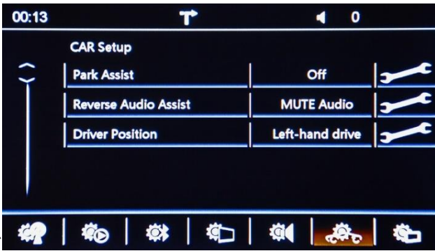
In Car Setup you can program the Zenec for reverse camera and other important settings
